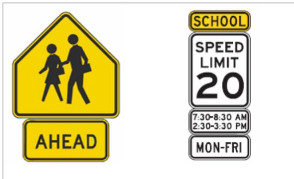
The location of the existing advanced warning signs satisfy the MUTCD standards. The location of the existing reduced speed limit signs are inconsistent with the MUTCD guideline (100' from the school property line). In most instances the "school speed limit 15" signs are posted between 50' and 225' from the school property or on school property itself. These deficiencies are noted in Figure 7.
