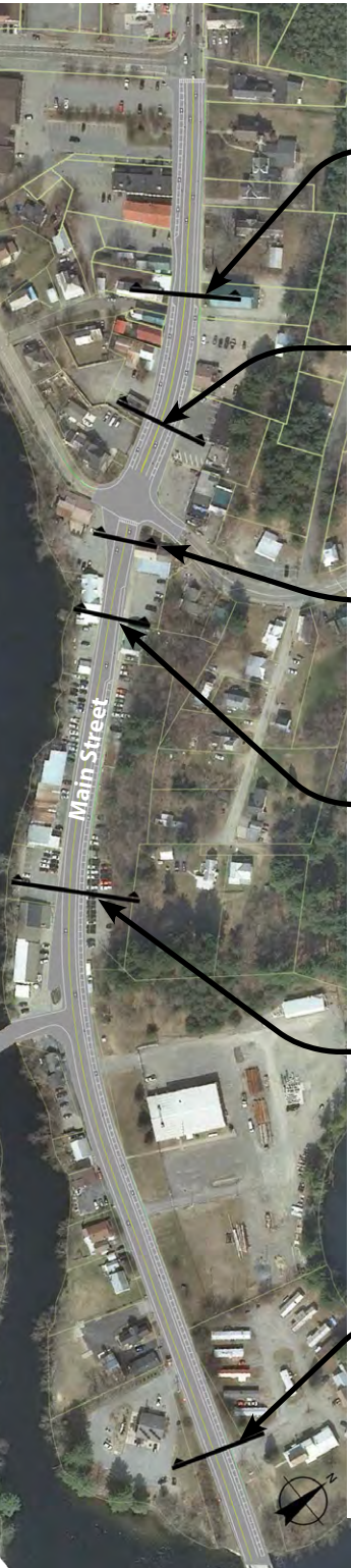
56' road width, 11' travel lanes, 5' bike lane (both directions), 7' parking lane (both directions).
