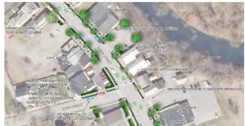
Examples of recommended access management and control recommendations to address large curb cuts (refer to Appendix B for full streetscape concept plan)
