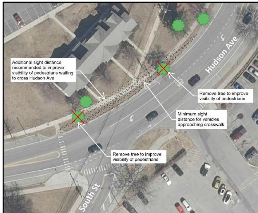
Figure 4-5: Recommended Tree Removals to Improve Sight Distance
