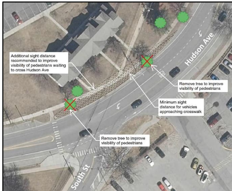
Figure 4-5: Recommended Tree Removals to Improve Sight Distance
