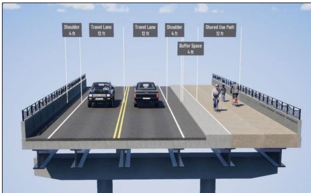
Figure 4-3: Recommended Bridge Section for Pedestrian and Bicyclist Accommodations
