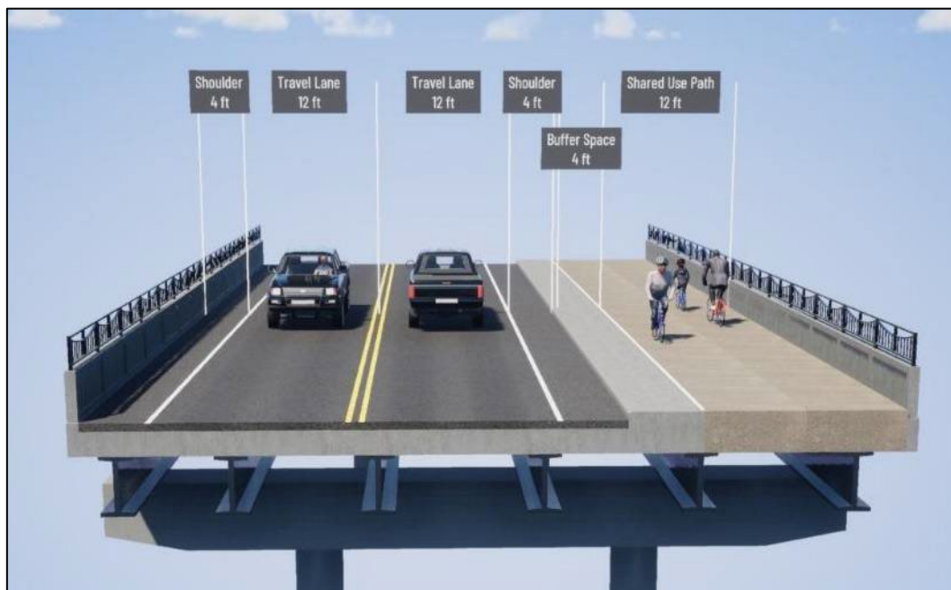
Figure 4-3: Recommended Bridge Section for Pedestrian and Bicyclist Accommodations
