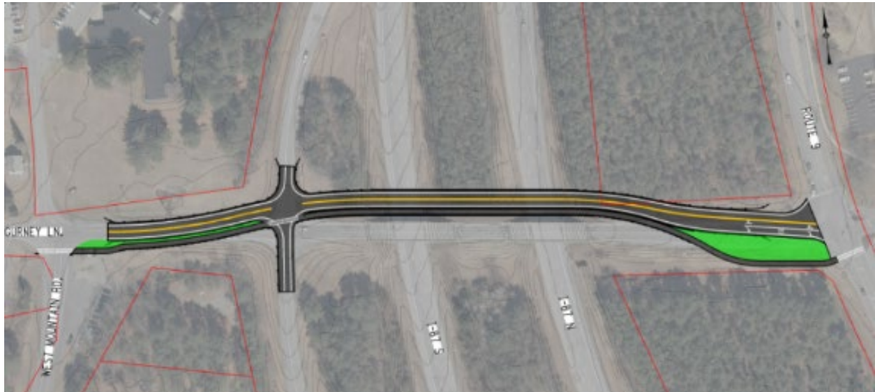
Figure 4-4: New Bridge Concept with a sidepath on the southern side of the realigned Gurney Lane
