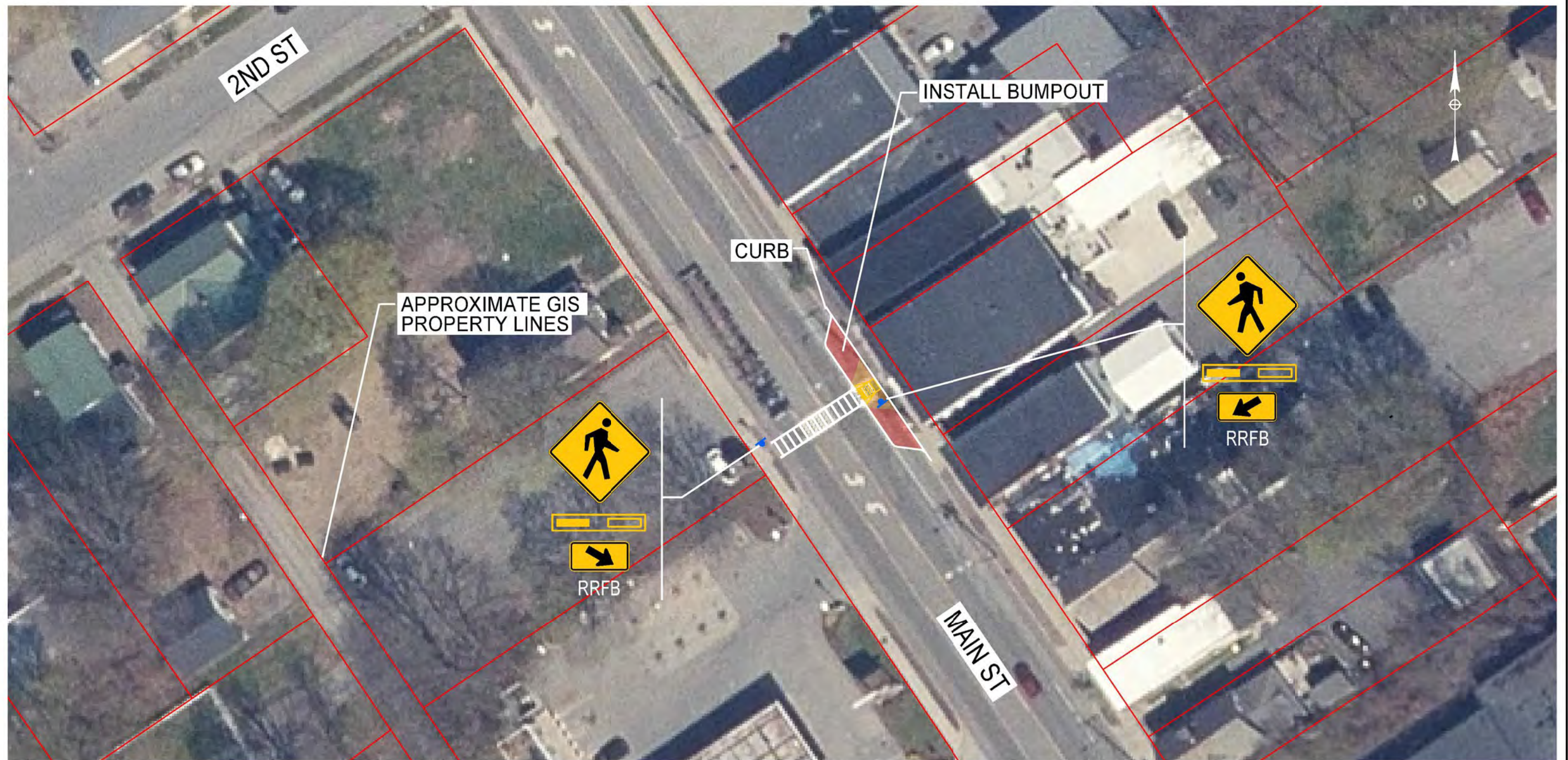
CONCEPT 2 - MID-BLOCK CROSSING, RRBF, AND BUMPOUT LAYOUT ON MAIN ST OPTION WITH CURB BUMPOUT
